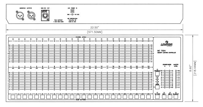
The MC 7000 Series lighting consoles are simple and flexible with three operating modes. These consoles provide standard 2-scene preset operation, single scene wide mode for double channel capacity and memory scene operation mode.
