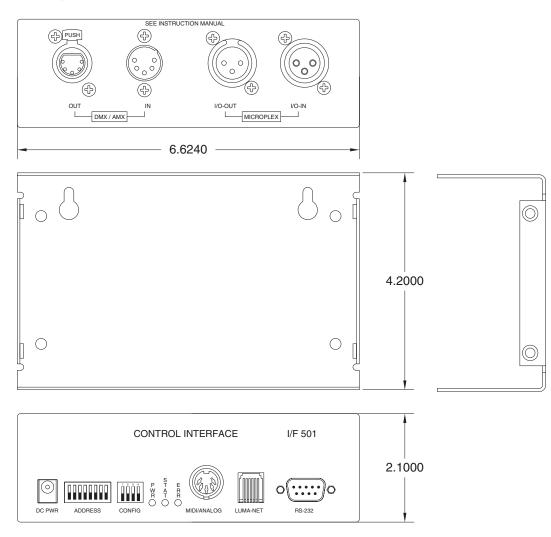
The Leviton-NSI IF 501 Control Interface is your simple solution for dimmer and control systems compatibility. Increased flexibility of control system design is achieved with the multiple signal ports and protocols available with the IF 501. The IF 501 may be configured to combine and convert analog, analog multi-plex and digital control signals.
